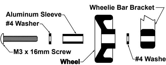
of the two wheelie bar brackets. Now install the screw assembly through the wheels and into the wheelie bar bracket in exactly the following order - M3 x 16mm buttonhead screw/ #4 washer/ aluminum sleeve/ **RPM** Wheel/ #4 washer/ **RPM** Wheelie Bar Bracket/ 3mm locknut. **Caution: The smooth, flat side of the #4 washers should face towards the wheel.**
