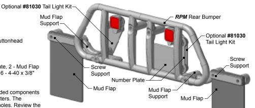
illustration to the right for proper position and placement of the Number Plate on your *RPM* Rear Bumper. Using 2 - 4-40 x 3/8" buttonhead screws, secure the Number Plate to the bumper. *Caution: Do not over tighten the screws!*
