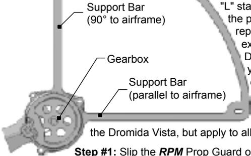
**Step #1:** Slip the *RPM* Prop Guard over the top of the gearbox and orient it so the support bars of the Guard point straight out of the front (or rear) of the airframe and 90° to the side.
