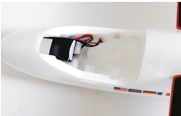
9. Position of the LiPo battery in the cabin.
