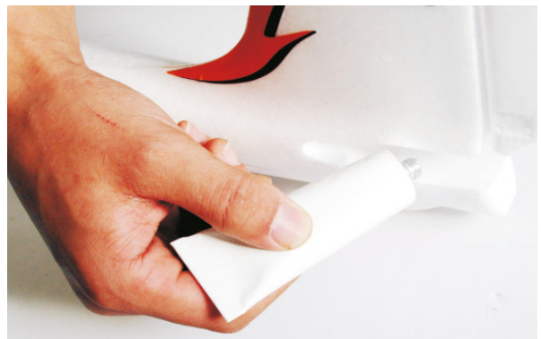
5. Apply glue to the contact surface on the fin. Note details on gluing further back in the instructions.
