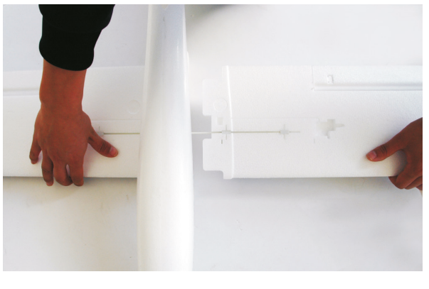
3. Insert the right wing half into the fuselage.
