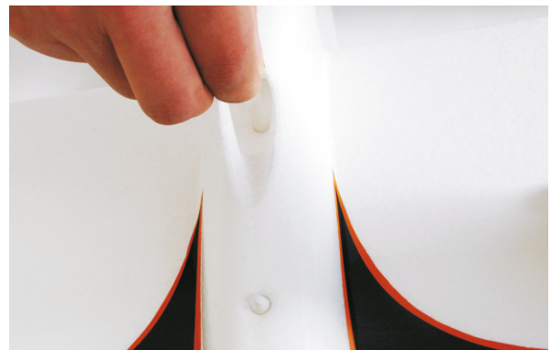
4. Secure the wing with the two plastic bolts.
