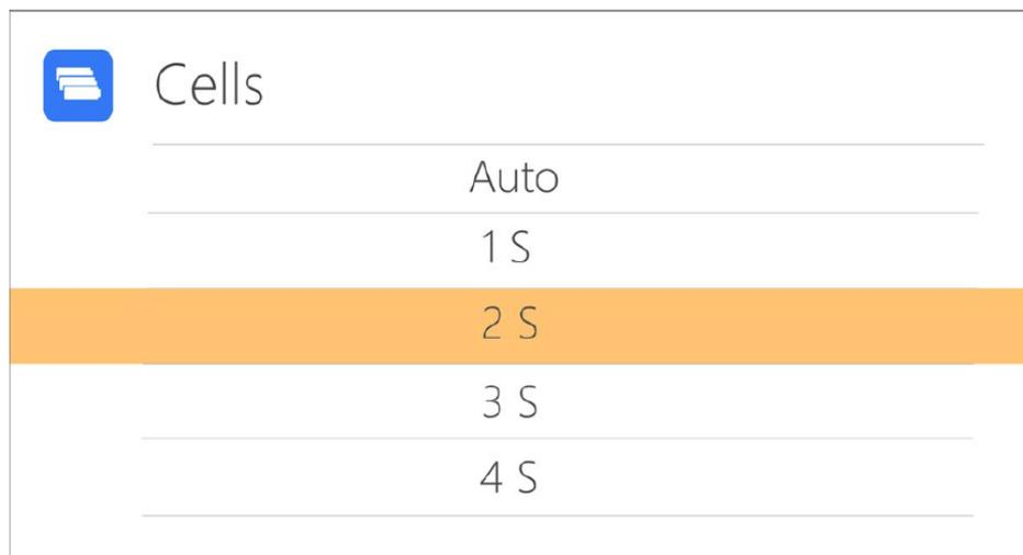
Scroll [Scroll Wheel] to adjust the value. When set to "Auto", the charger will automatically identify the number of cells connected to the battery according to the battery voltage connected to the output port. Short press [Scroll Wheel] and [CH/Exit] to take effect and return to the previous interface.
