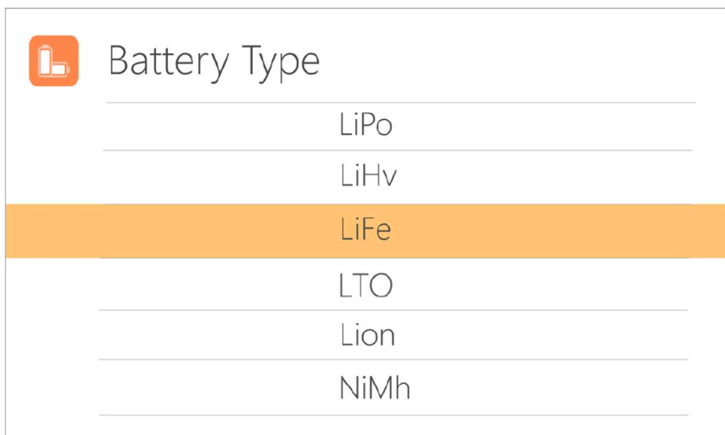
The charger supports Lipo, LiHV, LiFe, Lion, NiMh, PB chemistry batteries. After choosing the correct battery type, Short press [OK] and [CH/Exit] to take effect, and return to the previous interface.
