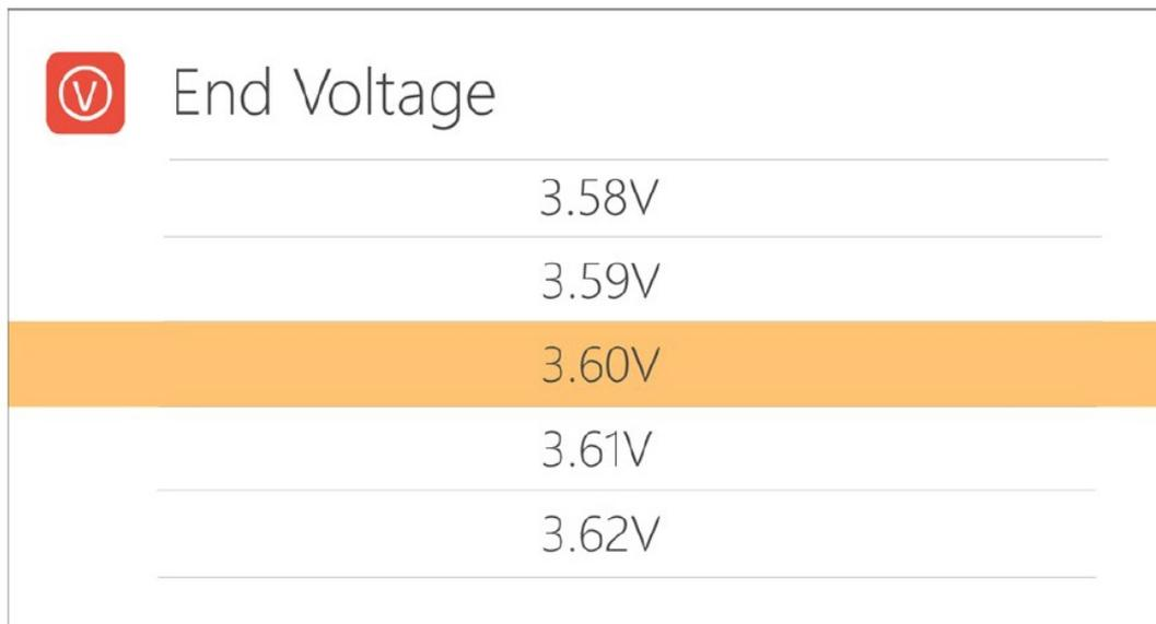
1. Only LiPo, LiHV, LiFe batteries can set the cut-off voltage.
