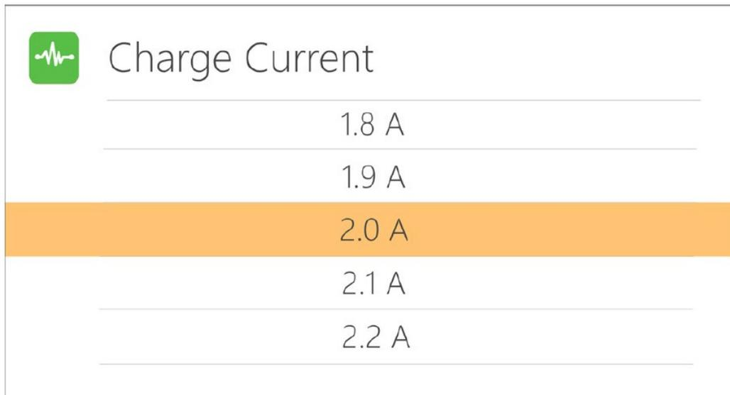
**Tips:** Please set the charging rate of 1-2C according to the battery capacity. For example, if the battery capacity is 2000mAh, please set the charging current to 2.0-4.0A. Check the guidelines of your battery's manufacturer for correct charging instructions.
