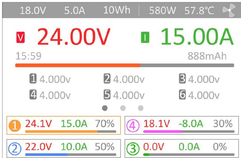
Scroll [Scroll Wheel] on this interface to switch the display of the internal resistance voltage value of the corresponding channel. Short press [Scroll Wheel] to dynamically set the working current or stop working. As shown below:
