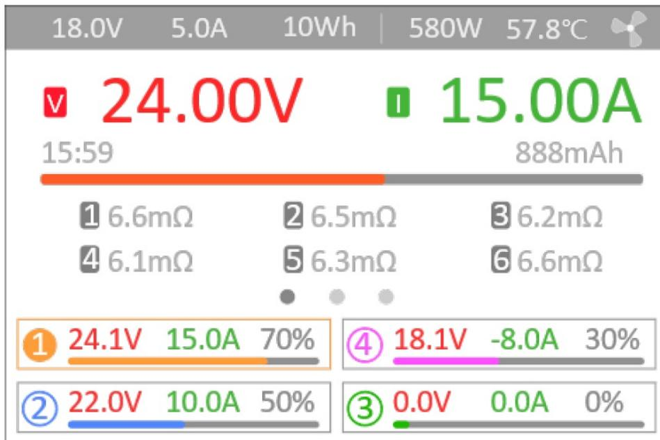
1mΩ: Internal resistance of the first battery
