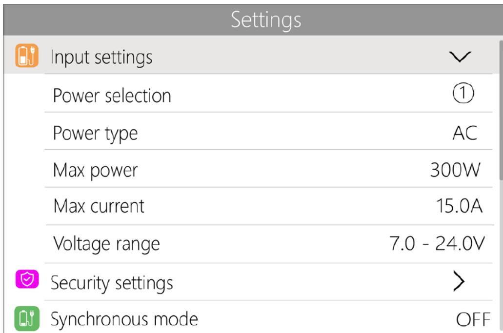
**Power selection:** When the AC power supply is connected, the power selection will be fixed to PI, power, current, and voltage are also fixed values. P1 and P2 can be selected when the input is DC. Users can set power, current, voltage by themselves.
