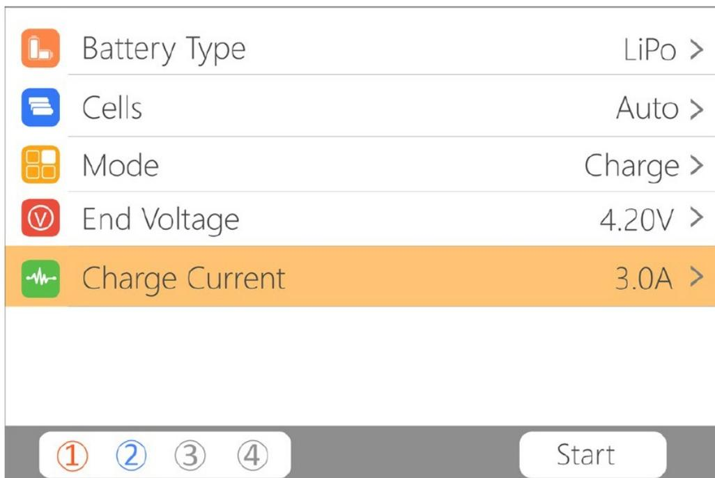
Move the cursor to “Battery Type” and short press [Scroll Wheel] to modify the battery type, the display is as follows:
