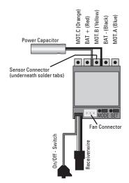
Receiver Connecting Wire: the Comet is equipped with an Nosram Multicon receiver wire. As supplied, it will easily fit in all ordinary receivers. Make sure you connect it to receiver with correct polarity and use channel 2.
