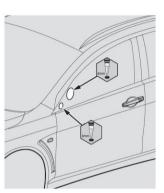
We recommend using our body reamer to drill mounting holes.
