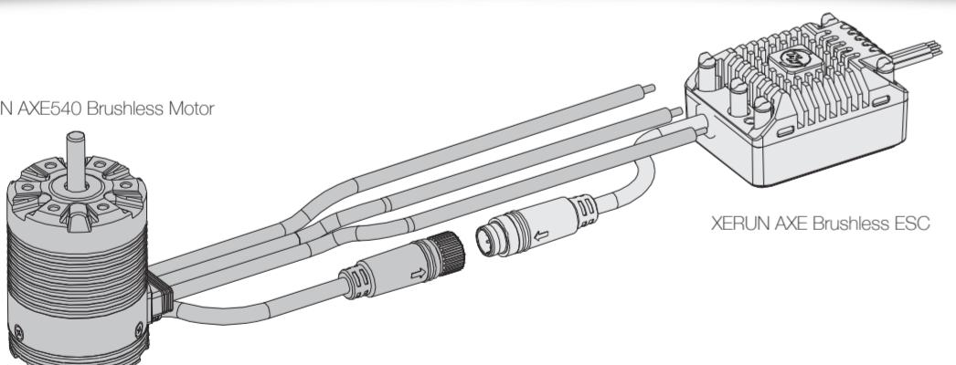
This is an extremely powerful brushless motor system. For your safety and the safety of those around you, we strongly recommend removing your pinion gear before performing calibration and programming functions with this system, and keeping wheels in the air when you turn on the ESC.
