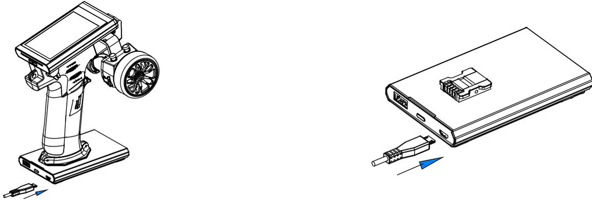
▶ The transmitter base can be charged directly by connecting the USB data cable.
