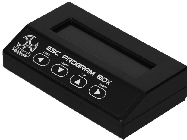
Optional ESC Program Box #ORI65202 available for advanced setup and firmware upgrade.
