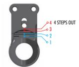
STEP 4 gives the least Ackermann and creates a lot of steering into & out of corners. However, the car is more difficult to drive in chicanes because there is less traction and stability.
