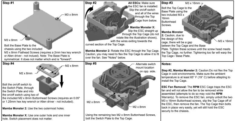
Alternate Mounting Options: The RPM ESC Cage is very versatile and can be mounted almost anywhere given enough space to drill & tap two 3mm mounting holes and fit the Base Plate in the area desired.
