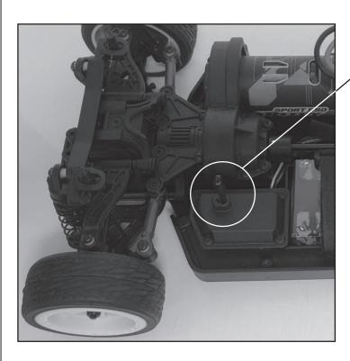
Install antenna wire through antenna tube, then install antenna / tube as shown.
