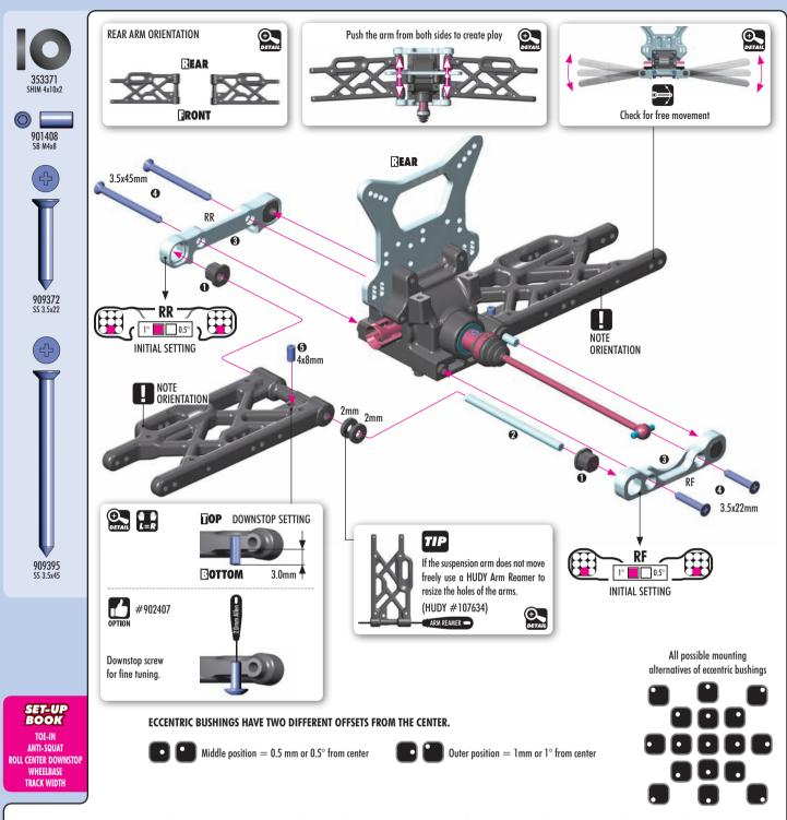
The XRAY rear alu lower suspension holders provide even greater range of adjustment for the rear suspension. Using different combinations of eccentric bushings, fine adjustment of rear anti-squat, rear toe-in, rear roll center, and rear track-width can be obtained. For more information about the influence of rear anti-squat, rear toe-in, rear roll center and rear track width on car handling, please refer to HUDY Off-Road Set-up Book (#209099).
