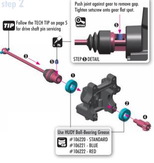
**BEFORE** inserting the clip on the central CVD shaft joint, apply a small amount of threadlock on the area where the clip goes.
