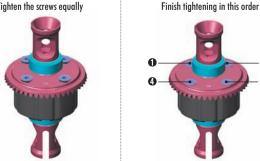
After assembly the differentials should have a length of 32.3 $\sim$ 32.5 mm measured from the ends of the installed ball-bearings. If differentials are longer, retighten the 4 screws holding the crown gears.
