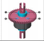
After assembly the differential should have a length of 32.3~32.5 mm measured from the ends of the installed ball-bearings. If differential is longer, retighten the 4 screws holding the spur gear.
