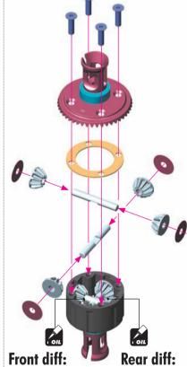
Silicone oil 5 000cSt Fill just above the satellite gears.
