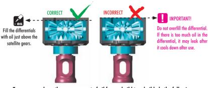
To ensure you have the same amount of oil from rebuild to rebuild, do the following:
