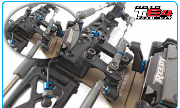
New adjustable height steering system. T6.2 is not adjustable
