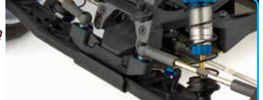
New 22.5 kickup and bulkhead options. T6.4 offers: 20.0, 22.5 and 25.0. T6.2 offers: 25.0 and 30.0.
