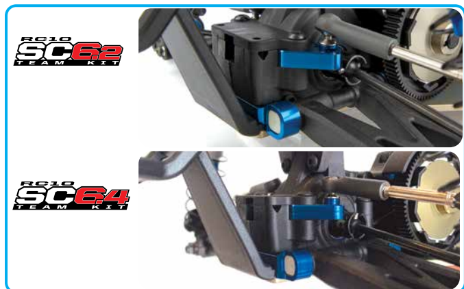
Updated CVA driveshafts, C and D mounts. SC6.4 offers: 92.5mm shafts and wide C and D mounts. SC6.2 offers: 91mm shafts and narrow C and D mounts.
