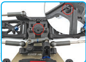
Keyed top plate to steering bellcrank brace
