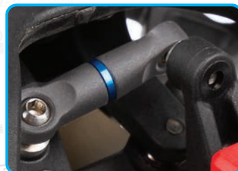
New material steering linkage rod ends
