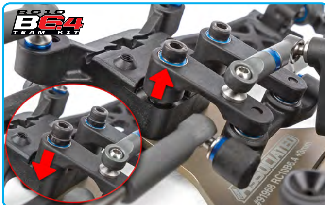
New adjustable height steering system. B6.3 is not adjustable
