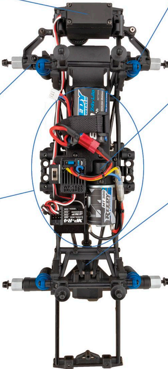
Includes 2.4GHz XP transmitter, receiver, Reedy Power water-resistant speed control, 380 motor, servo and 850mAh Li-Ion battery
