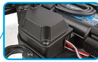
Water-resistant enclosed receiver box
