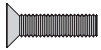
Z528 Flat Head Screw M3x12mm Senkkopfschraube M3x12mm Vis tête fraisée M3x12mm サラネジ M3x12mm
