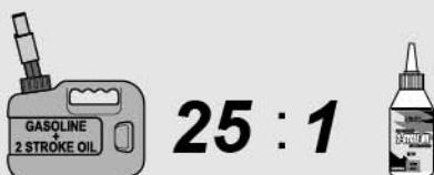
**Mixture Ratio of Gasoline and 2 Stroke Oil**
