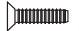
85260 Ⓞ TP. Flat Head Screw M2x8mm Flachkopfschraube Vis Tete Ronde T.Pサラネジ
