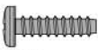
Z568 TP. Binder Head Screw M3x12mm Flachkopfschneidschraube M3x12mm Vis tole tête plate M3x12mm T.PバインドネジM3x12mm
