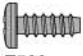
Z566 TP. Binder Head Screw M3x8mm Flachkopfschneidschraube M3x8mm Vis tole tête plate M3x8mm T.PバインドネジM3x8mm
