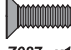
Z087 x1 Flat Head Screw M3x20mm Senkkopfschraube Vis tête plate サラネジ
