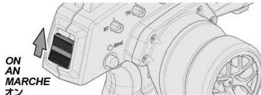
**3 Press and hold the receiver setup button, then turn the power switch to the ON position. The receiver LED will flash quickly. Release the setup button after 1 second.**
