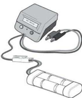
Only charge nickel cadmium (Ni-Cd) type batteries. Other types of batteries may burst causing injury or damage to persons and property. Do not charge batteries longer than recommended by your charger and battery instructions. Excessive heat can damage battery packs.
