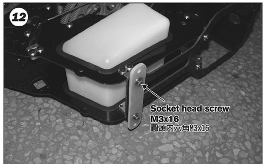
12 Fasten the spacers and fixing plate to the bottom plate with socket head screws M3x16 and washer \phi 3.4 \times \phi 9.9 \times \phi 0.9 \text{mm} . 以圓頭內六角螺絲M3x16與華司 \phi 3.4 \times \phi 9.9 \times \phi 0.9 \text{mm} 將墊片和固定片鎖附於底板。
