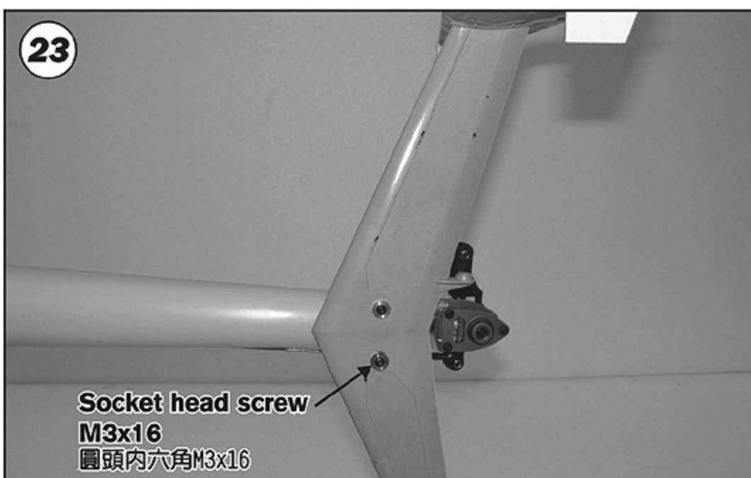
23 Fasten the vertical stabilizer with socket head screws M3x16 and washers. 裝上垂直翼，並以圓頭內六角螺絲M3x16與華司鎖緊固定。
