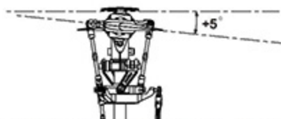
Stick position at Hovering/Throttle 70%/Pitch+5° 搖桿停懸/油門70%/Pitch+5°
