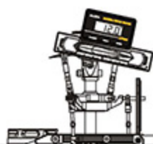
Stick position at high/Throttle 100%/Pitch+12° 搖桿高速/油門100%/Pitch+12°
