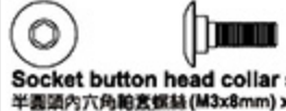
Socket button head collar screw 半圓頭內六角軸套螺絲(M3x8mm) x 12
