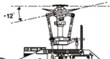
Stick position at low/Throttle 100%/Pitch-12° 搖桿低速/油門100%/Pitch-12°
