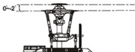
Stick position at low/Throttle 0%/Pitch0~2° 搖桿低速/油門0%/Pitch0~2°
