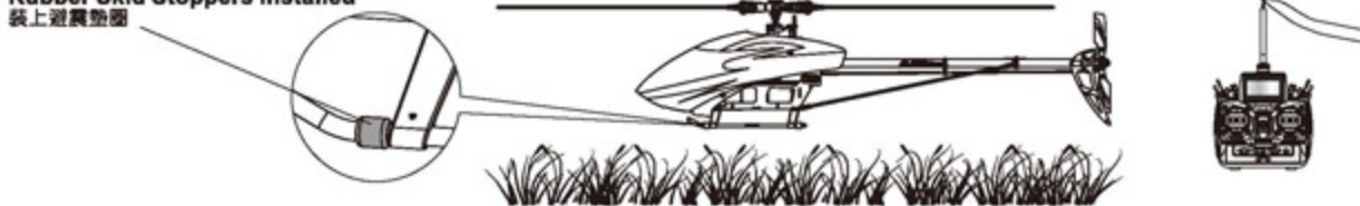
Rubber Skid Stoppers Installed 裝上避震墊圈
