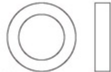
Bearing 軸承 (φ 12x φ 18x4mm) x 2
