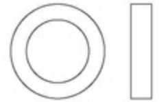
Bearing 軸承 ( \phi 12x \phi 18x4mm ) x 2
