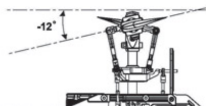
Stick position at low/Throttle 100%/Pitch-12° 搖桿低速/油門100%/Pitch-12°
