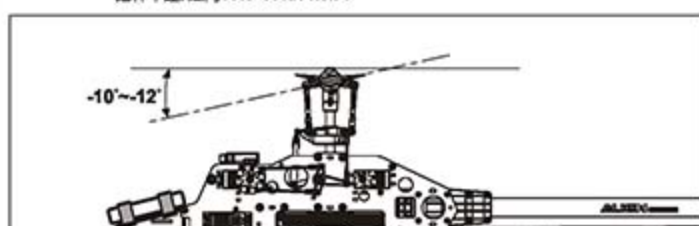
Stick Position at Low/Throttle 100%/Pitch -10°~+12° 搖桿低速/油門100%/Pitch-10°~+12°
