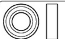
Bearing 軸承 (φ8xφ16x5mm) x 2
