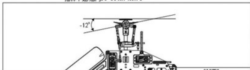
Stick position at low/Throttle 100%/Pitch -12° 搖桿低速/油門100%/Pitch -12°
