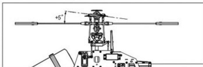
Stick position at Hovering/Throttle 60%/Pitch +5° 搖桿停懸/油門60%/Pitch +5°
