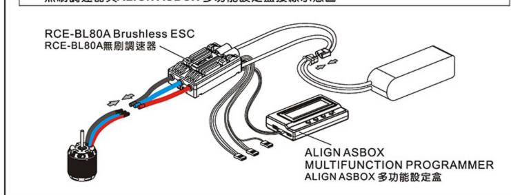
Apply another three-pin wire (with JR male connectors at both ends for connecting ESC and Multifunction Programmer. Plug the three-pin wire into ESC "-+P" port, and also plug into multifunction programmer "ESC" port.
