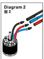
The motor rotates in different direction with different brand ESCs. If the wrong rotating direction happens, there are two ways to adjust it:
