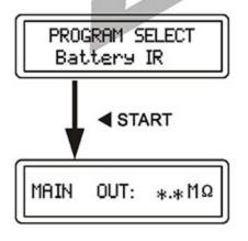
Measure the internal resistance of the battery to judge the quality of the battery
