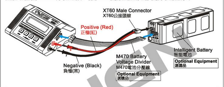
For single purchase RCC-100 balance charger, using XH balance board to charge lithium battery.
