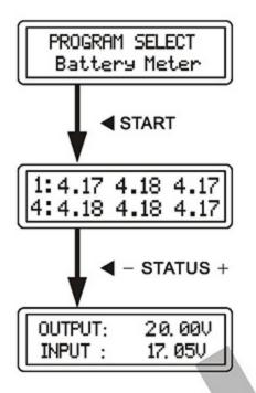
Measure a single voltage in the battery pack 可測量電池包内的單節電壓。
